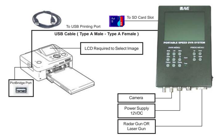
Figure 78: Connection Diagram between Digital Photo Printer and Portable Speed DVR System
