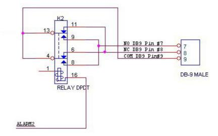
Figure 62: Hard Alarm Output Relay
