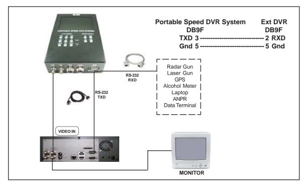
Figure 29: Portable Speed DVR System with External DVR Connections
